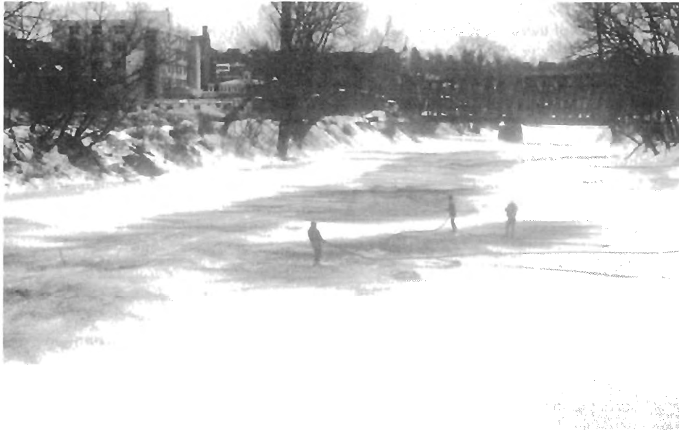
Figure 5. Site A after it was dusted (Montpelier, Vermont).
