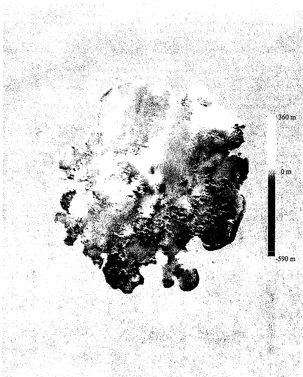
Figure 3. Comparison of the InSAR DEM with the rasterized elevation map from the University of Iceland Science Institute. The values shown are the InSAR elevations minus the University of Iceland elevations.
