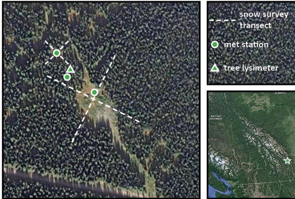
Figure 1. Layout of field site in the Canadian Rockies depicting the location of snow survey transects, three meteorological stations, and the tree lysimeter.
