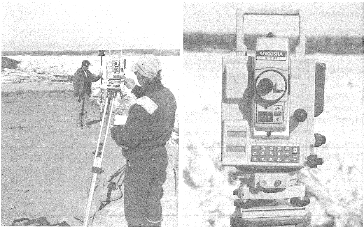
Figure 1 Digital theodolite, infra red electronic-distance measuring unit and on-board data acquisition system, positioned along the Liard River, N.W.T. Canada.
