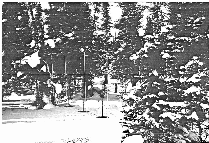
Figure 1. Set-up of snow temperature probes along a survey grid.
