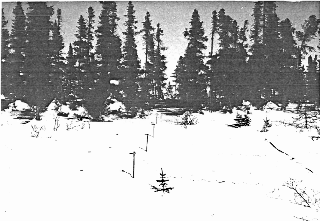
Figure 2. A radiometer transect extending into the forest canopy.
