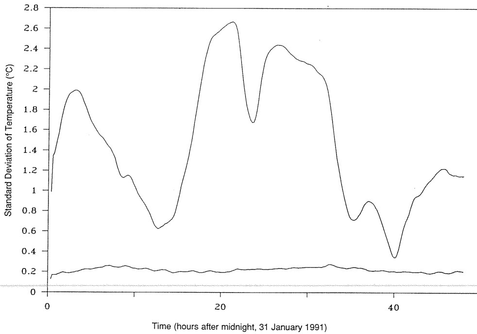
Figure 8. Standard deviation of snow temperature at mid-pack and at the snow/ground interface, as a function of time.
