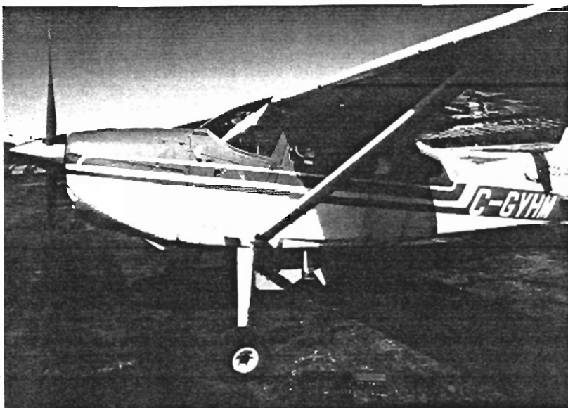
Figure 6. Camera pod mounted on Cessna 185.
