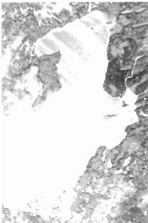
Figure 6. Reflectances on Crean Lake as derived from MAS data acquired on 8 February 1994. Higher reflectances are shown in the lighter grey tone and lower reflectances are shown in the darker grey tone.
