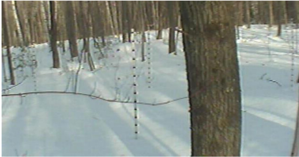
Figure 5. Snow stake photo taken daily by the Lorex Mcam: hardwood site shown here. Each of 15 thick black markers on the stake is made of 2 cm thick Duck Tape and marks every 10 cm interval for a total of 1.5 m. Snow depth was found by counting markers down from the top and estimating snow surface to the nearest 2 cm .
