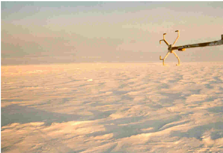
Figure 1. SHEBA sea ice in late October 1997, as seen from the 10-meter level of the Atmospheric Surface Flux Group 20-meter tower. The instrument is a sonic anemometer/thermometer.
