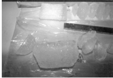
Figure 3. Ice core segment from 950 masl. Note that there is very little firn, suggesting that melt has taken place.
